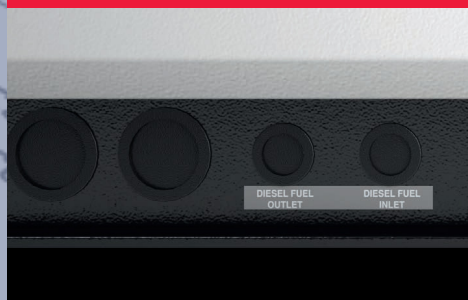
INPUT/OUTPUT FUEL PIPE
