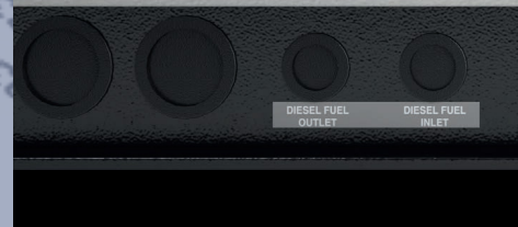
INPUT/OUTPUT FUEL PIPE
