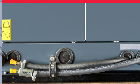
INPUT/OUTPUT FUEL PIPE
