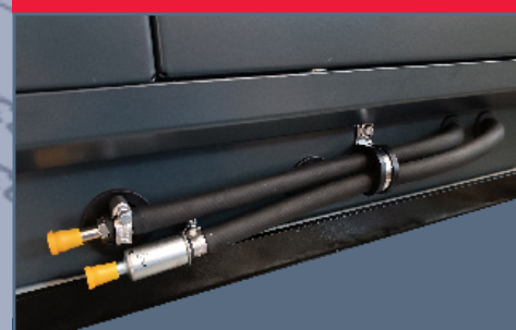
INPUT/OUTPUT FUEL PIPE
