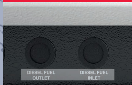
INPUT/OUTPUT FUEL PIPE
