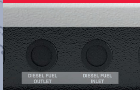
INPUT/OUTPUT FUEL PIPE
