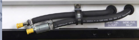
INPUT/OUTPUT FUEL PIPE
