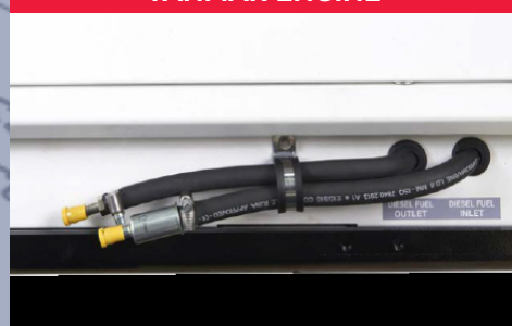
INPUT/OUTPUT FUEL PIPE
